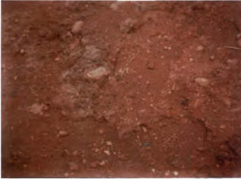
PLATE 10 : Close up shot in western Ajibode Primary School's area showing a section of cemented lateritic crust containing pebbles and gravels above cemented lateritic crust containing gravels only, at 7^{\circ}27'44''\text{N} and 3^{\circ}53'19''\text{E} . (Source: 2002 fieldwork)
