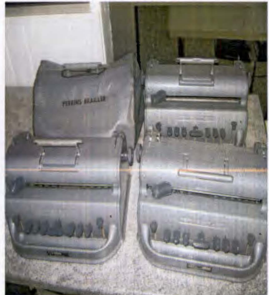
12. Perkins Brailier (writing device for the blind or visually impaired students)
